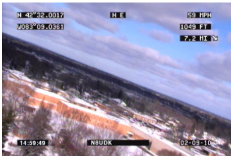
TV screen grab of the ID and GPS overlay from an in-flight R/C Aircraft showing Latitude, Longitude, Heading, Speed, Time, Altitude, waypoint DX and bearing plus Call letters from an OSD-GPS+ board.
