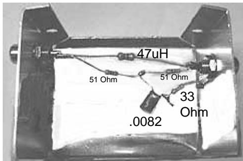
Twist one end of the 51 Ohm and .0082 uF leads together and then solder the parts as shown. Twist the other end of the cap with one end of the 33 Ohm resistor and solder together. Connect and solder the 47 uH to each RCA jack along with each end of the 51 Ohm resistors. Solder the 33 Ohm resistor lead to one of the ground lugs.
