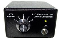
TVC-4S ATV down converter tunes 420-450 band to ch3 if you just want to try receiving but with more sensitivity than a cable TV set.
