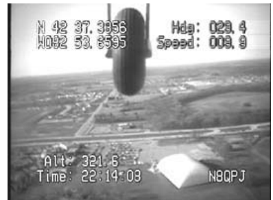
ATV from a R/C aircraft with GPS and call letter ID overlaid
