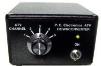
TVC-4S ATV down converter tunes 420-450 band to ch3 if you just want to try receiving but with more sensitivity than a cable TV set.
