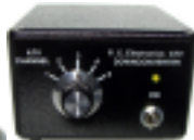
TVC-4S ATV Downconverter. 70cm to Ch3 $149
