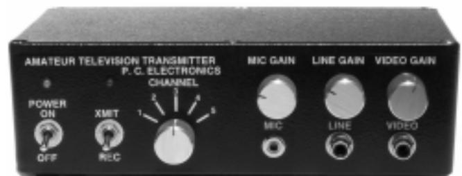
**VIDEO INPUT.** This input accepts any standard NTSC composite video into 75Ω from cameras, VCRs, computers, SSTV or RTTY converters, home satellite converters, etc. Use RCA phono plug and shielded cable (Radio Shack 15-1535) up to 12' or RG59 for longer runs. When unplugging, only twist clockwise to keep the jack from coming loose.
