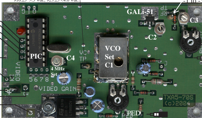
Blanking PEDestal pot Set for 60% P.E.P. To FMA5 sound board RG174 on bottom
