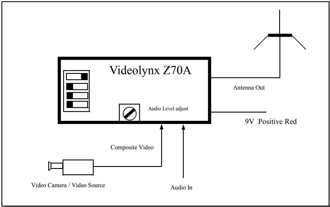
The diagram above shows how the **Z70A** needs to be connected to a video and audio source. Make sure that you have SMPTE standard video at 1 V P-P. Most consumer and commercial camera's and camcorders deliver SMPTE standard video, at the “**Video Out**” connector. If you are not sure if the camera is delivering SMPTE standard video, you can confirm this by looking at the video signal on an oscilloscope.
